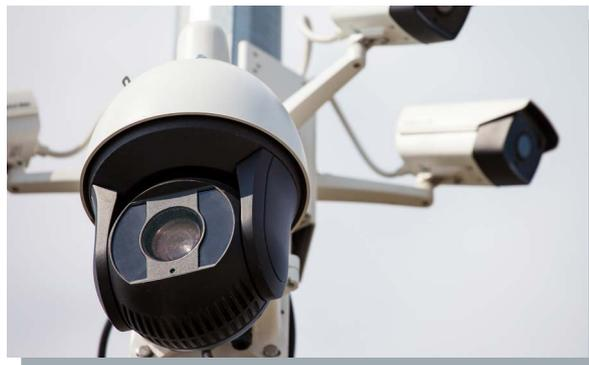
*Figure 4 and 5: Examples of Pan-Tilt-Zoom cameras*
